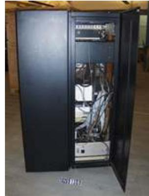
Gambar 4.6 Contoh Minicomputer PDP-8e Minicomputer System
